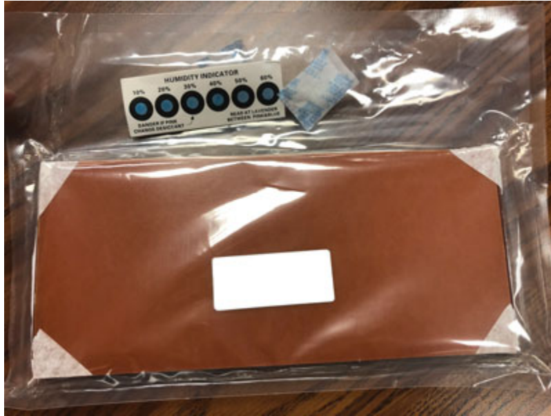
FIGURE 1. Including a desiccant pack and humidity indicator card (HIC) inside the sealed bag will help keep flexible circuits dry when they are on the shelf.
