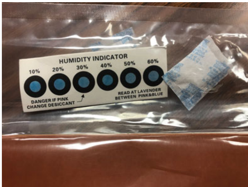
FIGURE 2. Close-up of the HIC.
