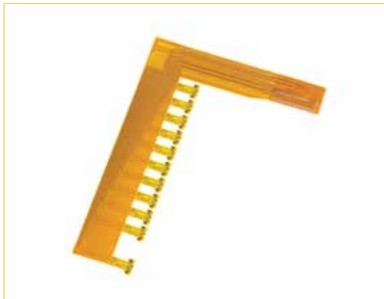
FIGURE 1. Copper planes can be cross-hatched to increase flexibility.
