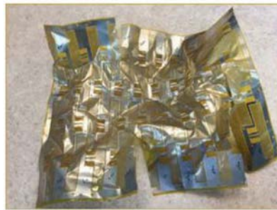
FIGURE 1. When panels get hung up in processing equipment, they are rarely salvageable.
