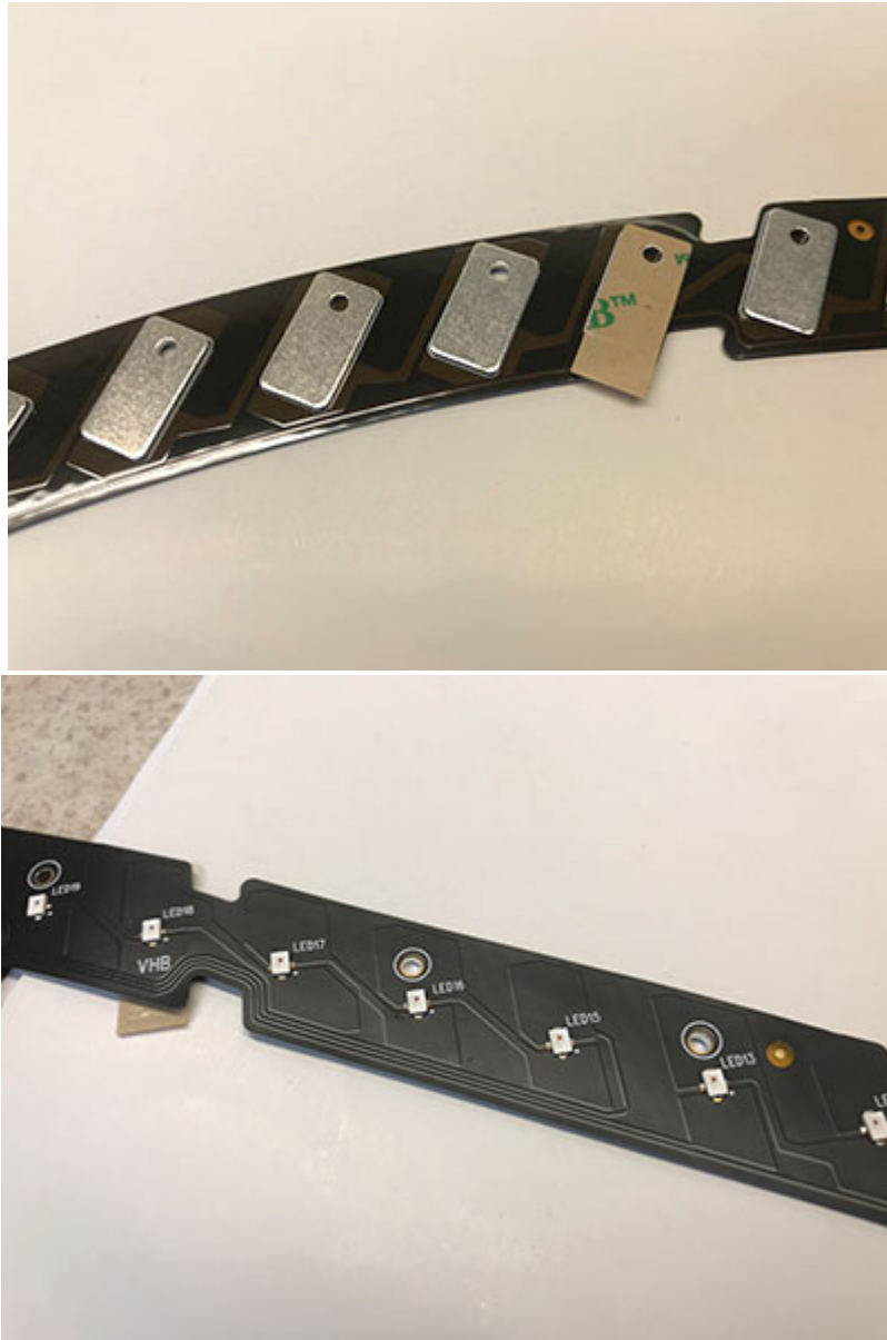
FIGURE 1. Aluminum stiffeners can be a great way to both stiffen the flex and dissipate heat from LEDs.
