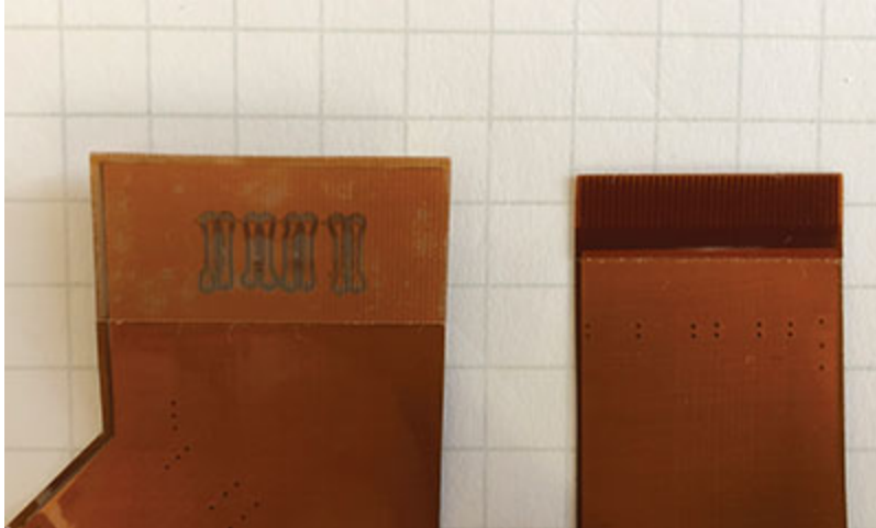
FIGURE 2. FR-4 (left) and polyimide (right) make up the lion's share of stiffener used today.
