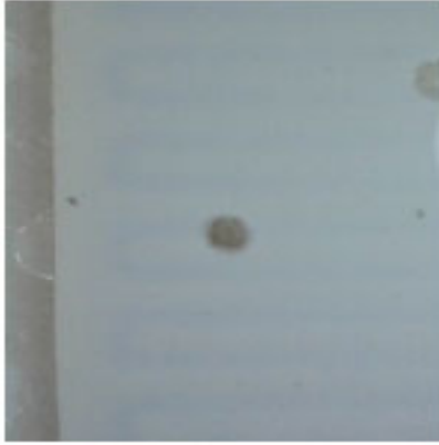
FIGURE 1. Adhesive specks on white polyimide following lamination.
