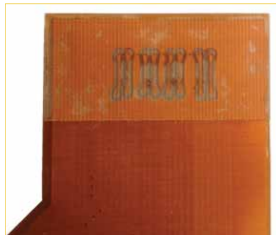
FIGURE 2. A stiffener bonded with pressure-sensitive adhesive. This adhesive is very effective, but will result in a few voids after lamination. These are mainly cosmetic and are not indicative of a poor or incomplete bond.
