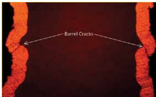
FIGURE 1. Barrel cracks most likely caused by low ductility copper plating.
