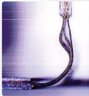
Potentially damaging forces can sometimes be reduced by unbonding layers in the bend area, as shown on the left. However, if the unbonded area is too short, buckling can lead to unacceptably tight bend radii as shown on the right.
